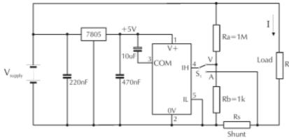
Measuring supply voltage and current to a load.  $S_1$  selects between voltage and current measurement. Ra and Rb shown scaled for  $200V_{FSR}$
