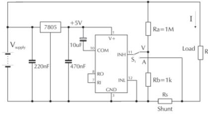
Measuring supply voltage and current to a load.  $S_1$  selects between voltage and current measurement. Ra and Rb shown scaled for 200V  $_{\rm FSR}$
